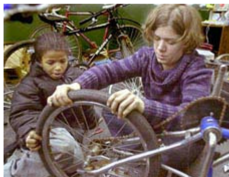
Devon Yates, right, works with Dereci Lowe, 12, on replacing a wheel and repairing brakes on a bike at Multi-Tool in Wilkinsburg. Yates volunteers for Free Rides, a bike recycling program that distributes working bikes and teaches bike repair. (Pam Panchak, Post-Gazette)
